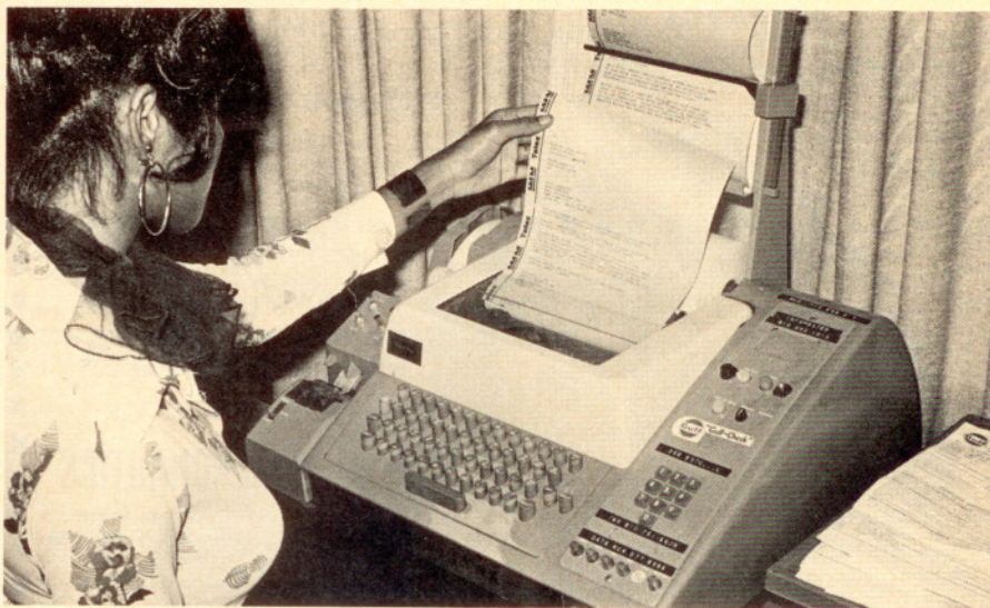
All used oil analysis data is typed into a master computer that diagnoses the engine's condition based on established wear patterns, previous history, and current test data.
